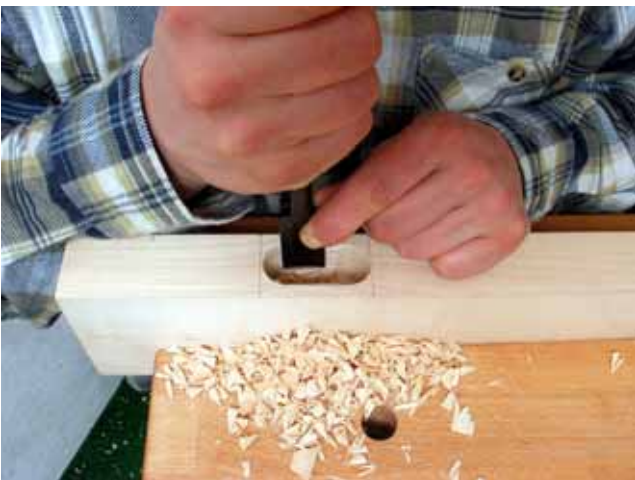
Cleaning up the cavity
