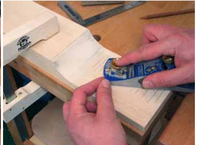
Removing material from the higher areas
