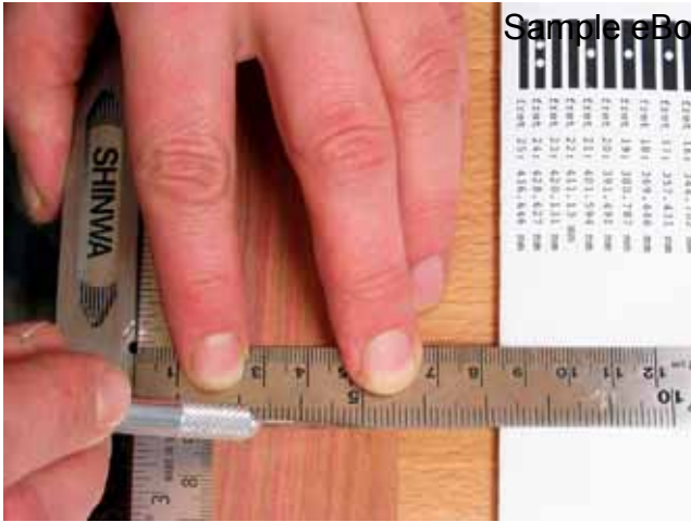
Marking the fret positions
