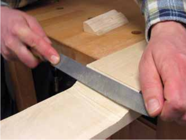
Smoothing the cut with a rasp ...
