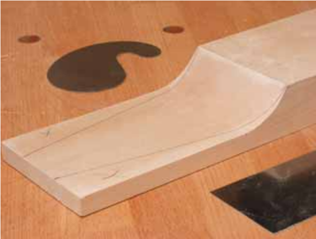
Only the area between the two lines has to be perfect
