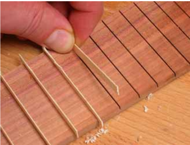
Inserting the maple veneer strips into the slots
