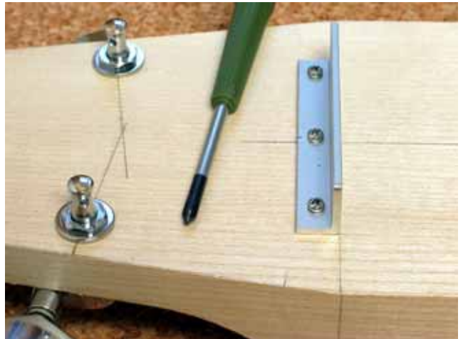
The nut is fastened centered and flush to line "B"
