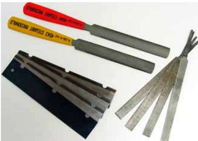
Nut files: the files on the left are actually small saw blades of different cutting widths
