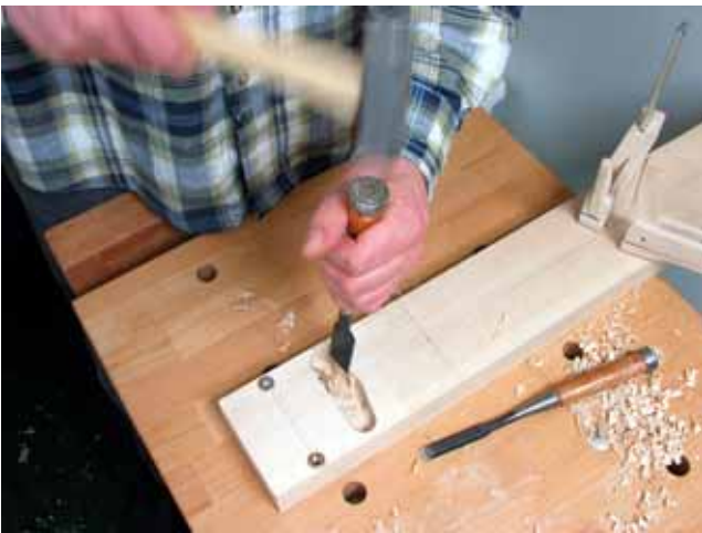
Removing the remaining material with a chisel
