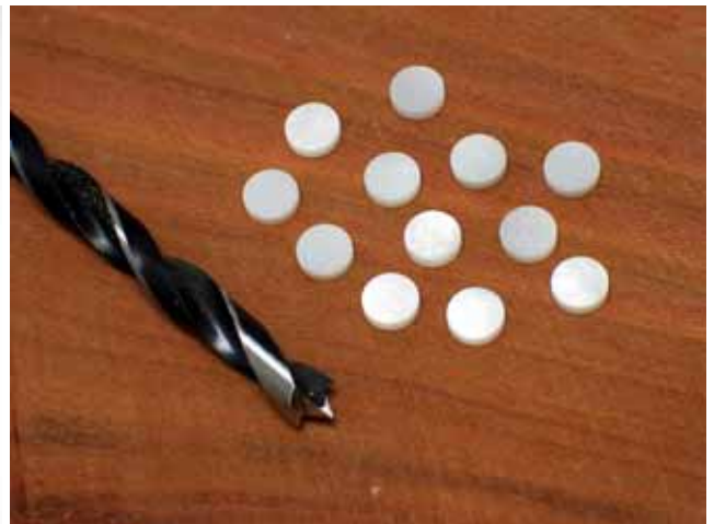
Inlay dots and brad-point drill bit of the same diameter
