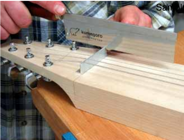
Cutting a notch for a string
