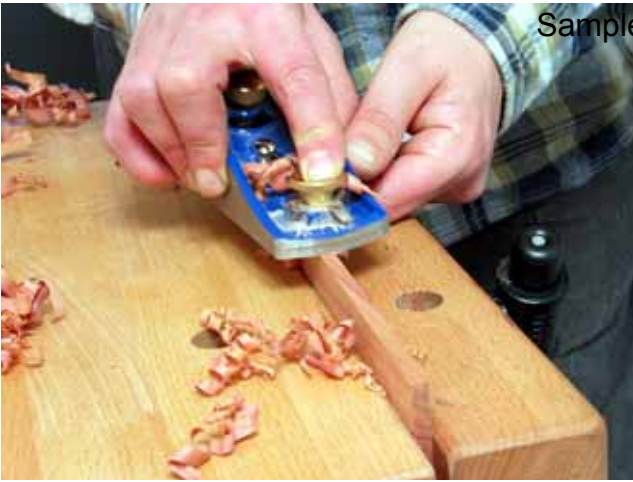
Plane one side of the fretboard blank dead-straight
