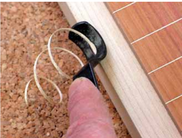
Veritas cornering tool in action
