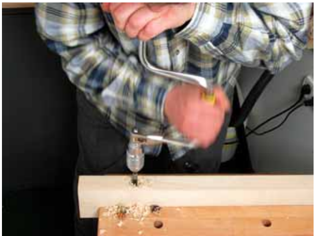
Pre-drilling the control cavity
