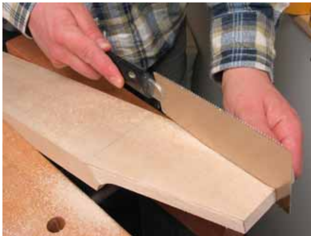
Cutting the peghead taper
