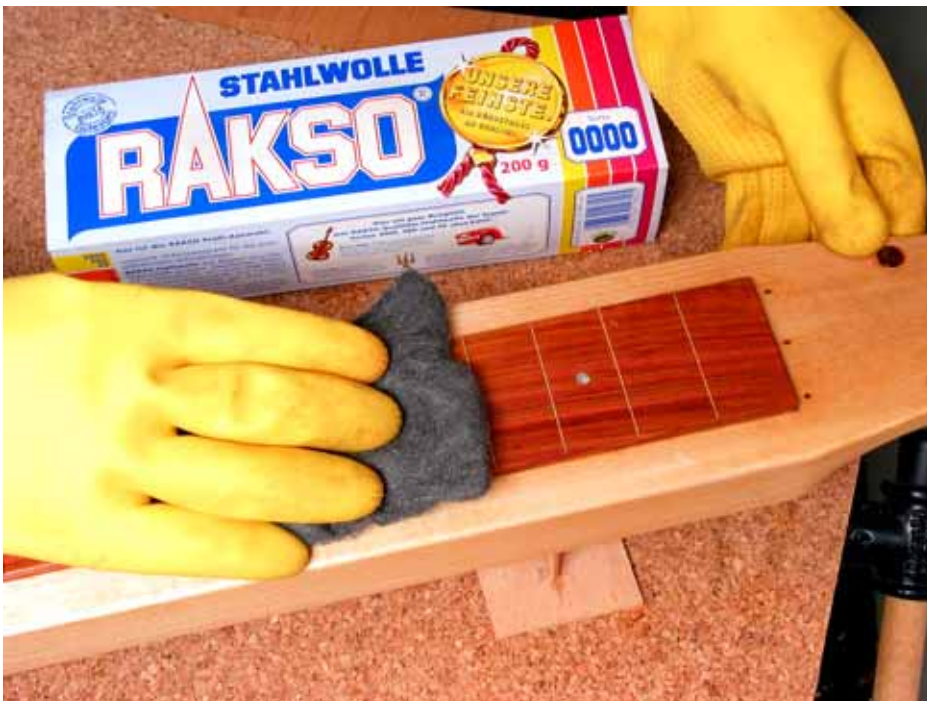
Rubbing the wet oil coat with steel wool
