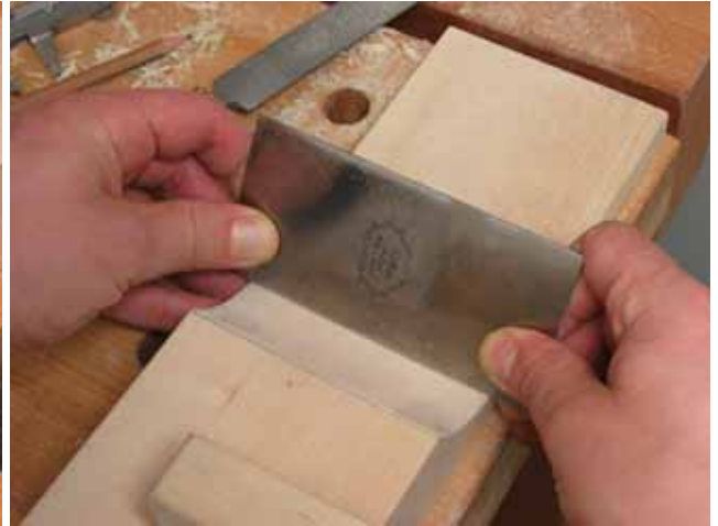
Final cleaning of the surface
