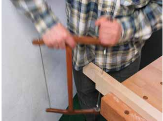
Cutting the concave transition
