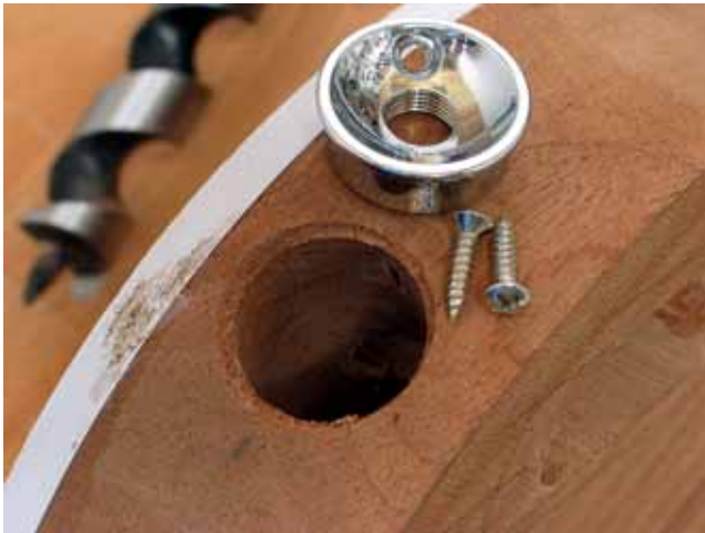
The output jack hole with jack mount
