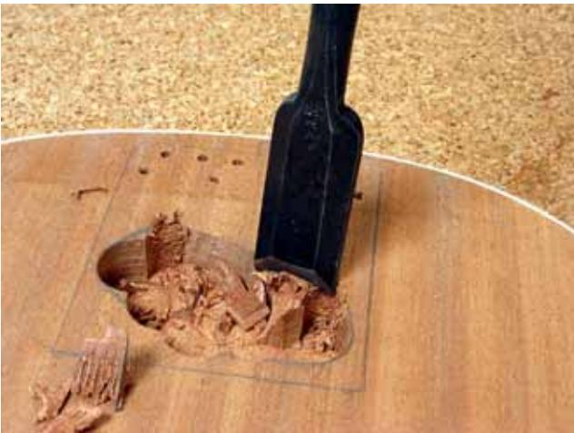
Removing material with a chisel
