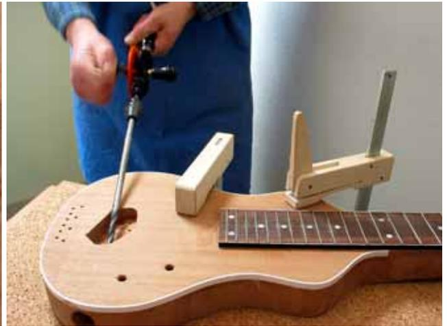
Connecting the pickup cavity with the control cavity
