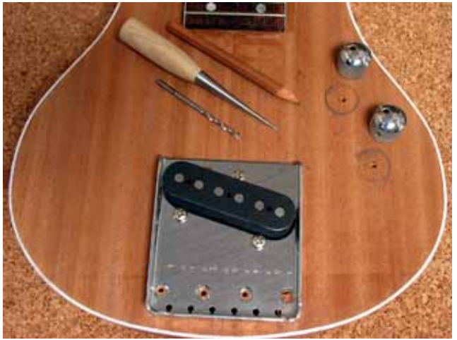
Marking the holes for the control pots
