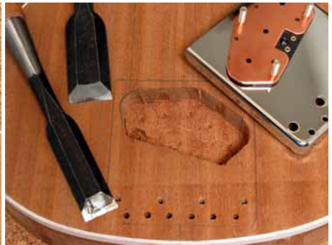
The finished pickup cavity
