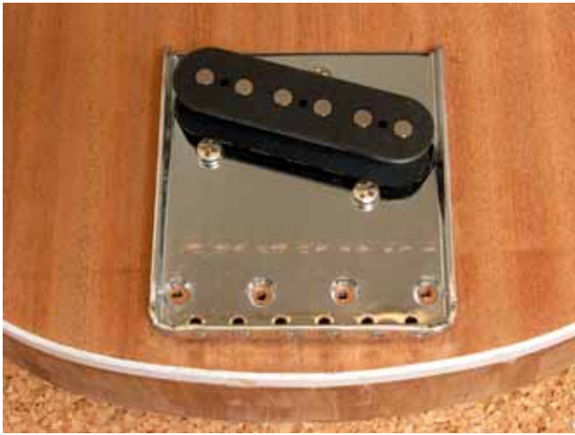
After mounting the bridge
