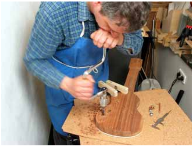
Pre-drilling the control cavity
