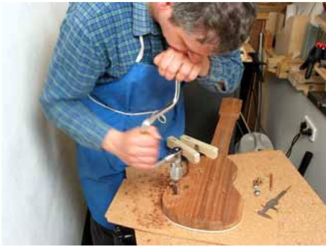
Pre-drilling the control cavity
