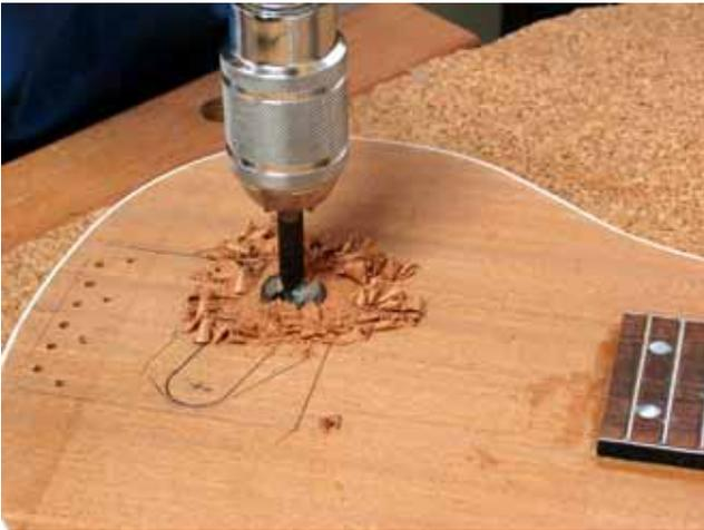
Pre-drilling the pickup cavity
