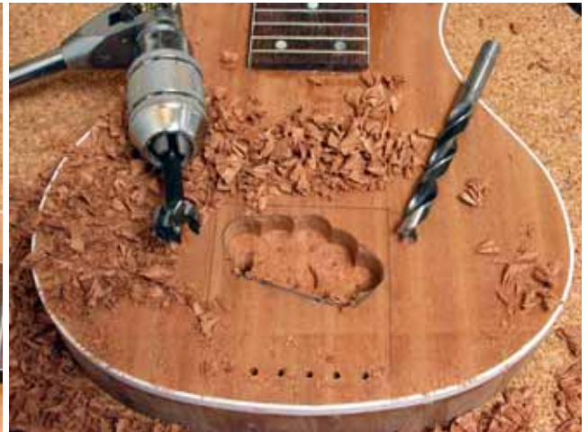
The pre-drilled pickup cavity
