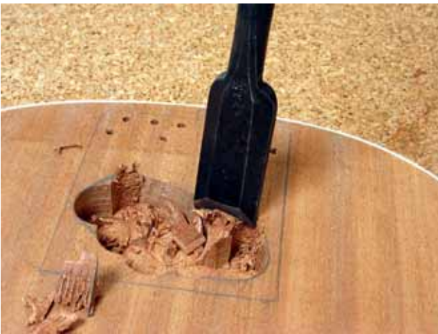
Removing material with a chisel
