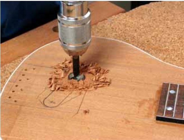
Pre-drilling the pickup cavity
