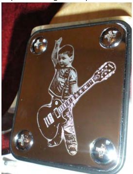
Neck plate custom engraved using impact engraving from a photo. This photo taken using the flash on the camera, but the actual effect on the real thing is very holographic – amazing.
