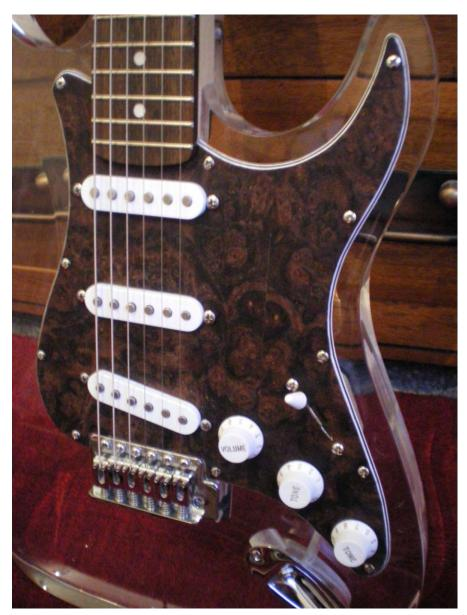
First attempt at laminating a scratch plate. Had to use 2 hour epoxy and make some mdf clamping cauls to hold everything flat while the glue went off. Walnut burr is awful to work with and it seems impossible to get it as flat as straight grain veneers before gluing, so this was the only way. The contrast between the walnut burr and the white of the scratchplate/hardware looks great.
